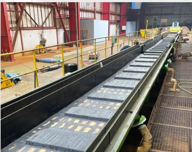
Assembly of the new pickling tubs on one of the two production lines
